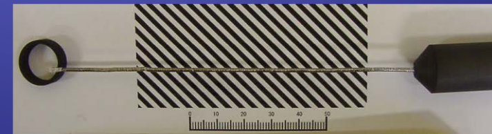
Fe-Ni-Ga alloy fiber produced from carbon crucible (right) with conically shaped bottom (Scale in mm)
