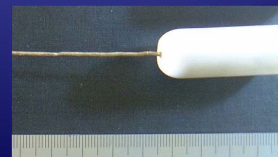
Cu 72 Al 17 Mn 11 alloy fiber produced from Al 2 O 3 ceramic crucible (right) with spherically shaped bottom (Scale in mm)
