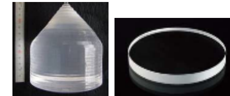
Fig. 1. LiCAF single crystal ingot (left) and disk (right) with 4 inches diameter.
